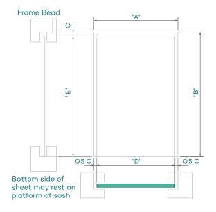
Figure 13: Thermal Expansion allowance of LEXAN sheet in the glazing profiles
