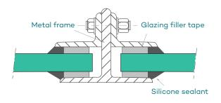
Figure 28: LEXAN sheet installation by using aluminum clamping profile
