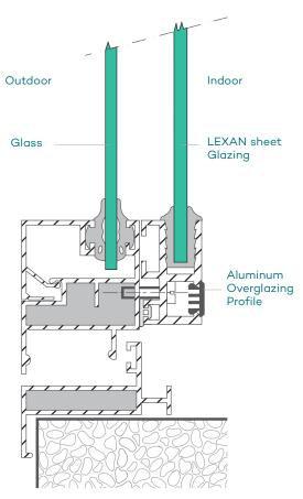
Figure 19: External Overglazing
